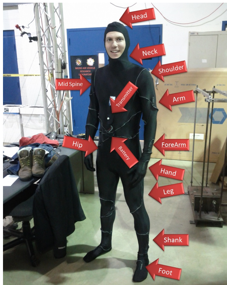
Figure 2.3: BPMS sensor locations and cables routing
