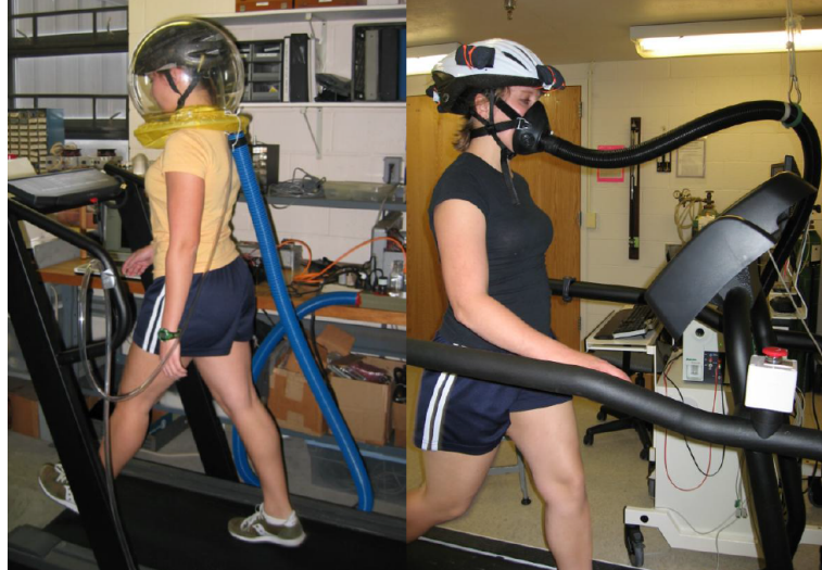
Figure 1.4: Metabolic workload measurement rig [67]
