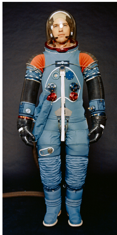
Figure 1.2: The A7L suit without the protective garments (TMG), source:NASA
