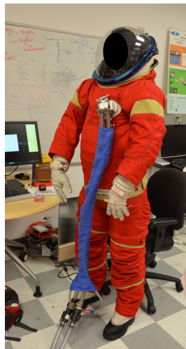
Figure 3.4: ILC Dover Launch and reentry I-Suit
