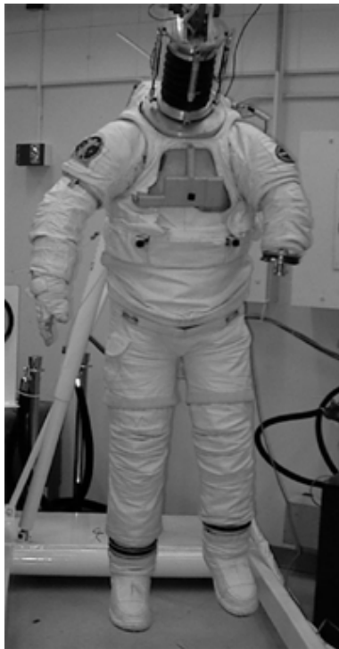
Figure 1.7: Robotic Space Suit Tester wearing the EMU [22]
