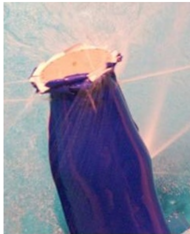
Figure B.12: Water Filled Pressurized Section: Leaks
