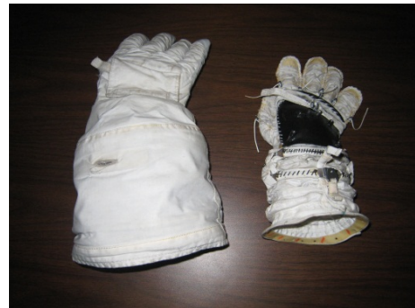
Figure A.3: Phase VI IMU glove and power-glove without TMG
