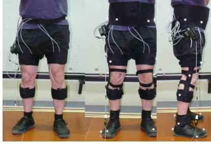
Figure 1.8: Inertial motion capture of the lower limbs and Vicon markers during a comparison study [41]
