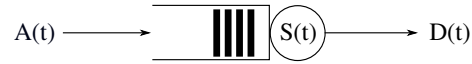
Figure 2: A queuing system that links the arrivals A(t) of a system to its departures D(t) by a service curve S(t) .
