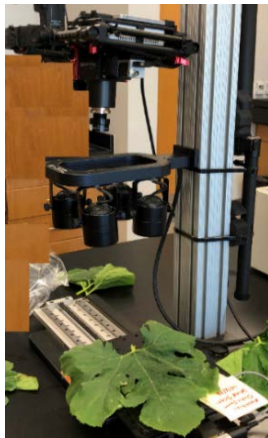
Figure 2: Laboratory spectral measurements of squash leaves using a benchtop hyperspectral imaging system.
