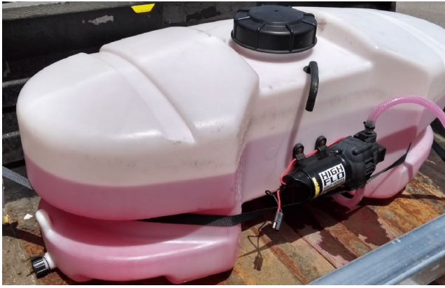
Figure 4. Tank and pump.
