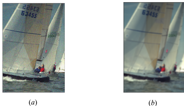
Fig. 3 Comparison of IQA algorithms on blurred and noisy images (a) noise image: subjective mean opinion score (MOS) = 44.7534, SSIM = 0.3491, MS-SSIM = 0.8539, 3-SSIM = 0.6120, 3-MS-SSIM = 0.9391 (b) blurred image: MOS = 66.3322, SSIM = 0.6932, MS-SSIM = 0.8825, 3-SSIM = 0.4933, 3-MS-SSIM = 0.8364.
