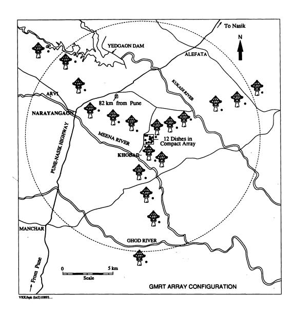
Figure 1. Antenna configuration of the Giant Metrewave Radio Telescope. The dotted circle indicates the approximate size of the synthesized aperture.
