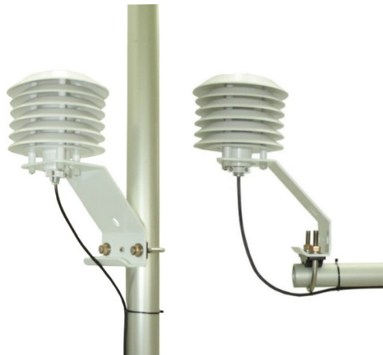
FIGURE 7-3. HMP60 and 41303-5A Radiation Shield on a tripod mast (left) and on a CM202 Crossarm (right)
