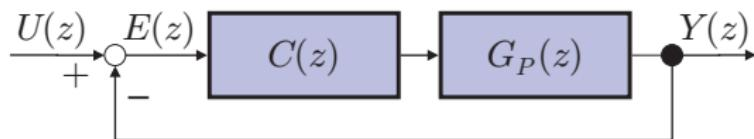
$$G(z) = \frac{Y(z)}{U(z)} = \frac{C(z)G_P(z)}{1 + C(z)G_P(z)}, \quad \frac{E(z)}{U(z)} = \frac{1}{1 + C(z)G_P(z)}$$
