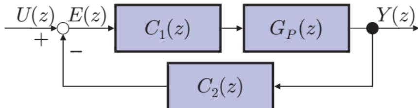
$$G(z) = \frac{Y(z)}{U(z)} = \frac{C_1(z)G_P(z)}{1 + C_1(z)C_2(z)G_P(z)}, \quad \frac{E(z)}{U(z)} = \frac{1}{1 + C_1(z)C_2(z)G_P(z)}$$
