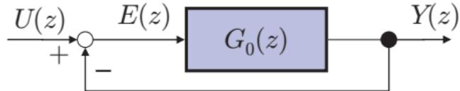
$$G(z) = \frac{Y(z)}{U(z)} = \frac{G_0(z)}{1 + G_0(z)}, \quad \frac{E(z)}{U(z)} = \frac{1}{1 + G_0(z)}$$
