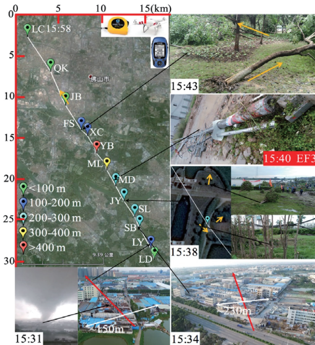
Fig. 8. Damage path, funnel cloud photo, and pictures from the ground damage survey for the tornado that formed in an outer rainband of the landfalling Typhoon Mujigae (2015). The damage path width is also indicated in the damage path figure. Adopted from Zhao et al. (2016).
