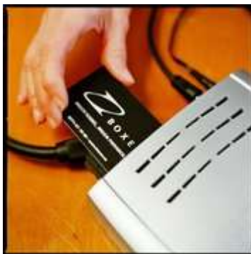
Decryption cards like this are needed in order to view certain digital TV stations in Sweden.
