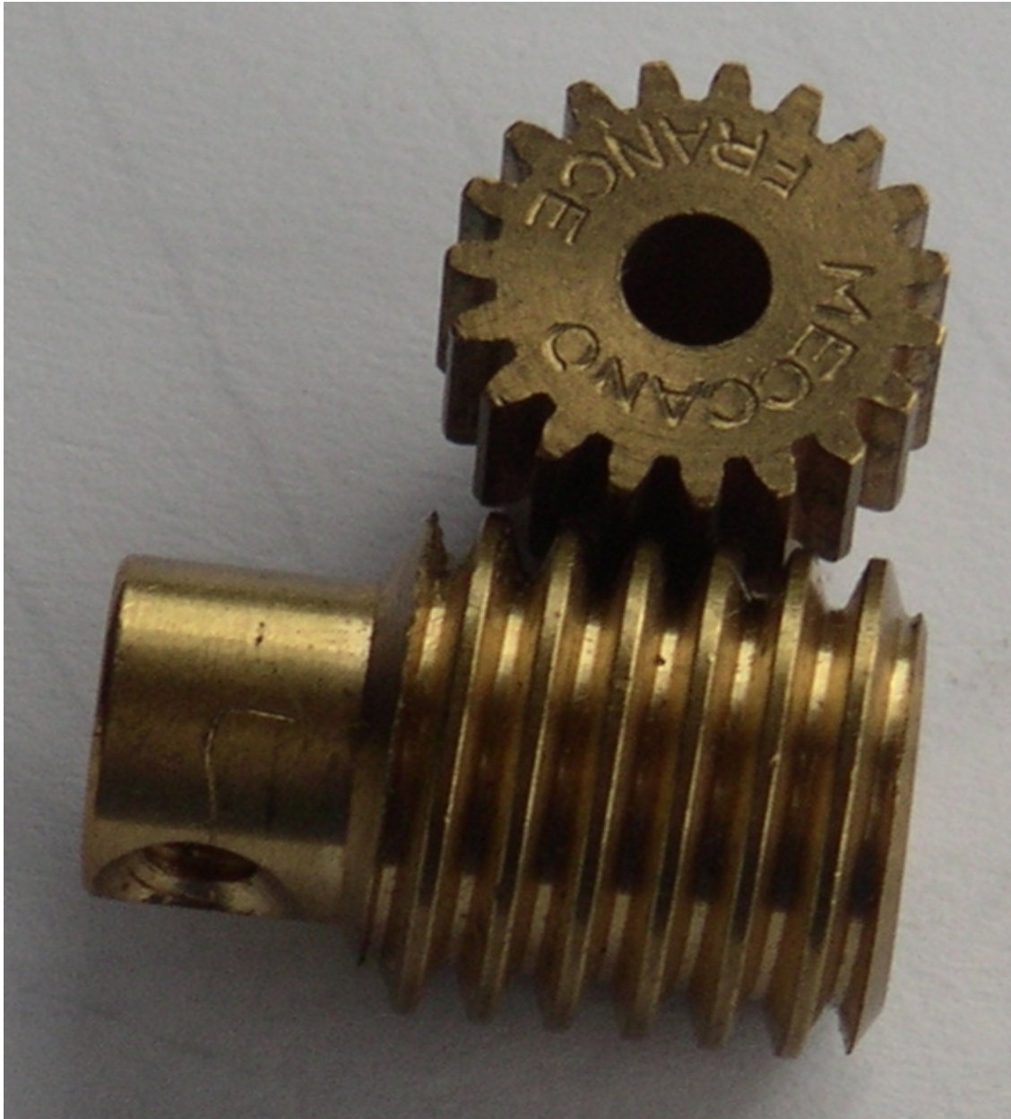
Figure 11 An Example of a Worm Gear and Pinion
