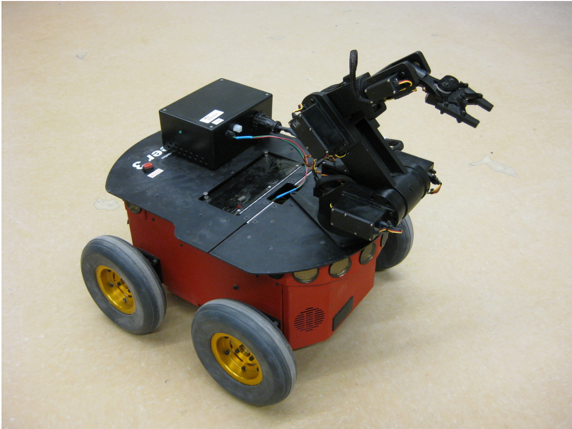
Figure 60 The Pioneer 3-AT robot has four motors and four unsteered wheels; on each side a pair of motors drives a pair of wheels through a single belt.
