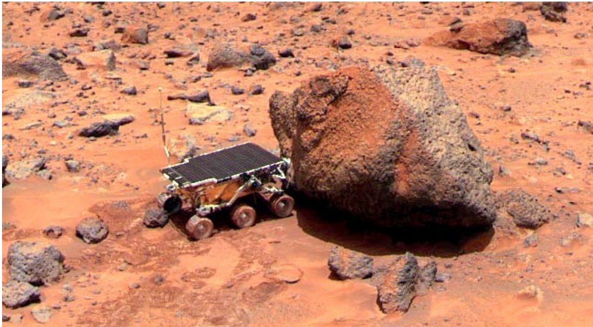
Figure 51 Sojourner taking an X-ray measurement of Yogi.
