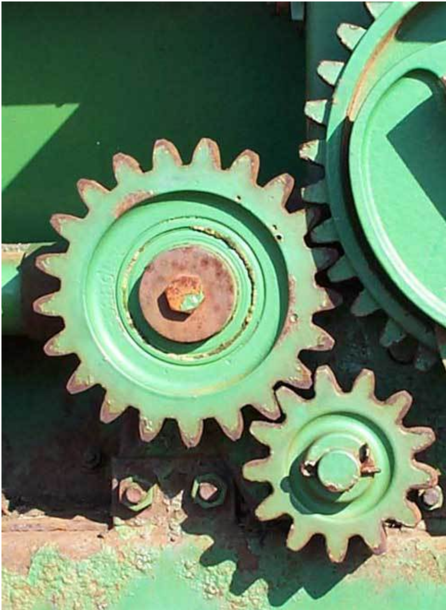
Figure 10 Spur gears found on a piece of farm equipment
