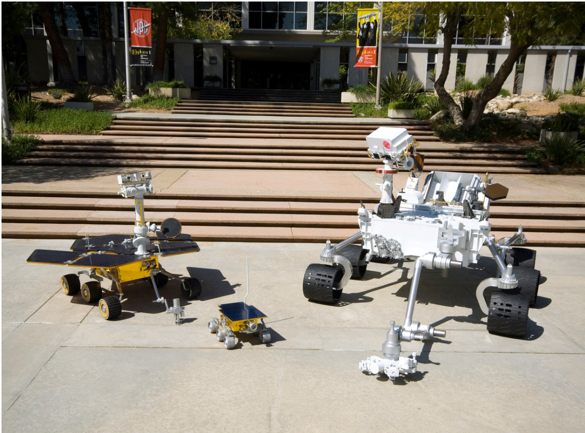
Figure 49 Mars Science Laboratory mockup (right) compared with the Mars Exploration Rover (left) and Sojourner rover (center)
