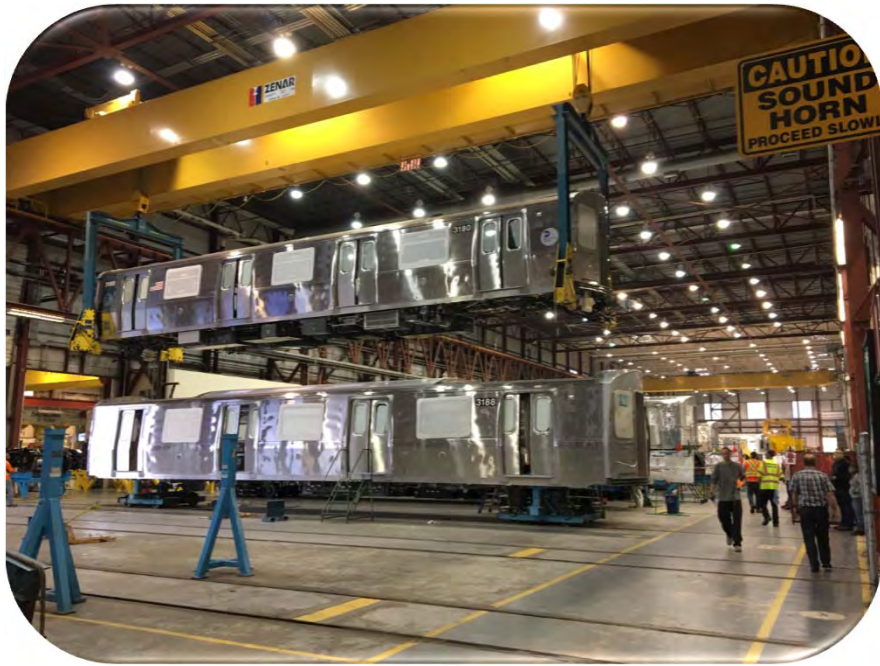
R179 car being transported from Station 14 (Car Shell Sealing) to Station 15 for water testing.
