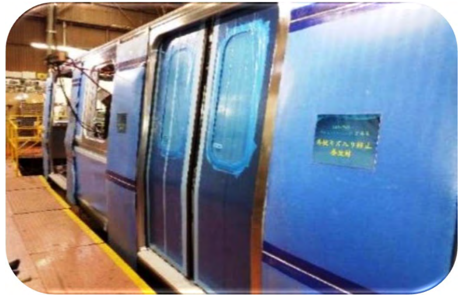
Side Panel with doors installed
