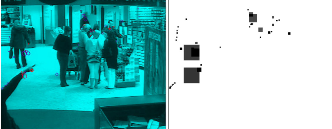
Figure 5: Example of a Pointing frame with learned compound features shown as circles (left) and corresponding probability map (right) where dark means high probability.
