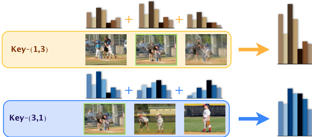
Fig. 3: Each video is represented by the sum of the BoW histograms extracted from multiple keyframes.
