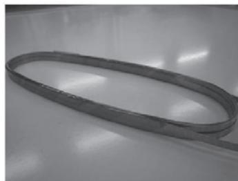
Fig. 1 Photograph of a DI-BSCCO<sup>®</sup> coil for stator windings.
