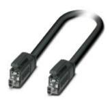
Patch cable, type: IEC 63171-2, degree of protection: IP20, cable length: 2 m, number of positions: 2, 1 Gbps, connection method: Crimp connection, connection cross section: AWG 22- 22, Single Pair Ethernet
