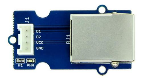
The Grove-RJ45 Adapter is a module which can convert a standard Grove connector to a RJ45 connector. Universal 4-Pin Grove cables can not meet the requirements when Arduino remote connect and control Grove module. Through two RJ45 adapter and a cable, It is able to achieve communication between Arduino and Grove
