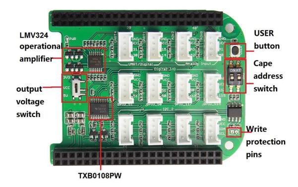
**Output voltage switch**, is a switch to control output voltage to Grove ports.
