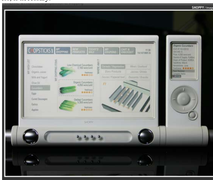
Fig. 14: The big device is for the shopping cart, while the small portable version is for user. Theme: From menu preparation to shopping. (Source: KAIST for Project “Chopsticks”)
