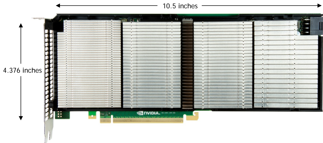
Figure 2. NVIDIA GRID K1 Graphics Board Dimensions
