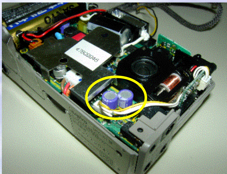
OS-CON 10SL47M(2p) Φ 6.3mm × L5.0mm
