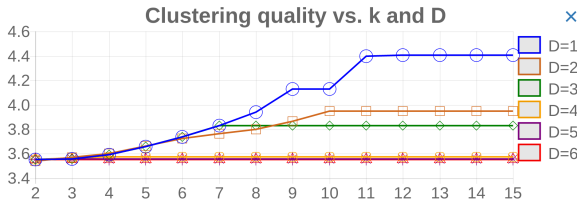
Figure 2: Visualization for parameter selection: how results vary for different k and D (some lines overlap).
