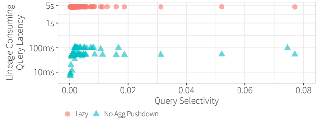
Figure 10: SMOKE-I reduces the lineage consuming query latency by 72.9 \times on average as compared to LAZY. With aggregation push-down, the latency is \approx 0 ms and we do not plot it.
