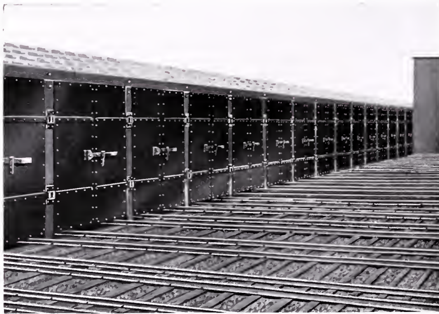
View showing a series of Swinging Sheet Tunnel Doors. Complete with hinges and improved relief spring latches. Mounted on steel Dryer front
