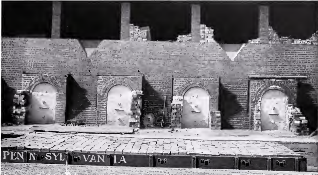
Showing Four Chambers Ahead of Fire. These Chambers are Water-Smoking with the Advancing Heat from the Burning Brick
