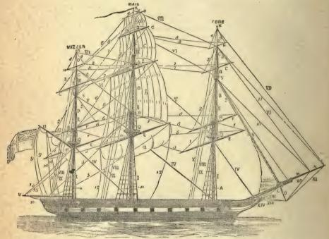
Spars, etc.—A, mast; B, topmast; C, topgallantmast; D, royal-mast; E, ; ard; F, topsail-yard; G, topgallantsail-yard; H, royal-yard; K, truck; L, bowsprit; M, jib-boom; N, flying jib-boom; O, martingale; P, chains; Q, top; R, cap; S, crosstrees; T, topmast cap; U, gaff; V, boom, or spanker-
