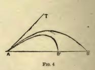
and of half the time of flight, or after it has traversed half its horizontal range; hence, by putting x=2h sin. A cos. A in equation II., or  $t=\frac{v\sin A}{h}$  in equation I., we obtain  $y = h \sin^2 A$ . A slight examination of the expression for the range will show that it is greatest when the body is projected upward at an angle of 45° to the horizon, and that a body projected at a greater angle than 45° has the same range as one projected at an angle correspondingly less (Fig. 3).
