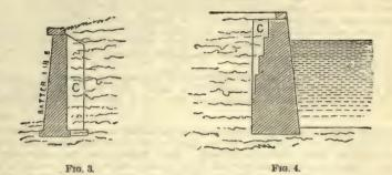
into a semi-fluid state, in which it gives a very much increased pressure on the wall. For this purpose, holes are left through the wall called "weeping holes;" these holes are about 9 in. high and 2 in. wide, and are generally placed about 1 for every 36 sq. ft. of wall. Also stones without mortar are frequently built up behind the wall, so forming an open stratum, into which the water drains, and is thence carried off through the weeping-holes.
