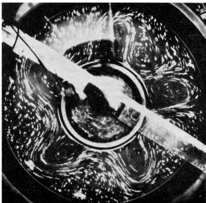
Fig. 10. In this experiment the water is heated from below at the rim of the rotating pan, and is cooled by means of a coolant at the center. The temperature contrast between the outer and inner side is in this case fairly small, while the rotation velocity (counterclockwise) is great. A symmetric circulation between the periphery and the center is no longer possible; a system of almost stationary horizontal waves forms which resemble in many particulars the long waves in the atmosphere (picture by D. FULTZ, University of Chicago).
