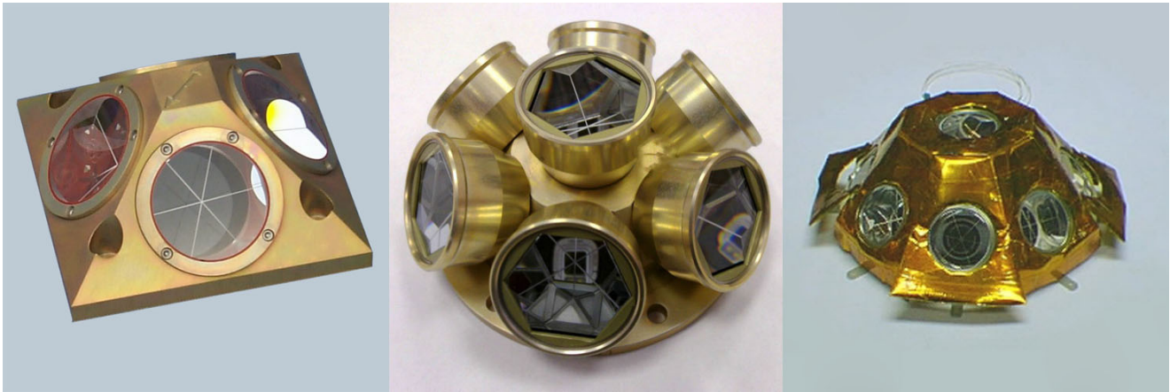
Fig. 1 Laser retroreflector array types used in various LEO missions. Left : CHAMP/GRACE/TerraSAR-X (courtesy GeoForschungsZentrum Potsdam); center : Sentinel-3 (courtesy IPIE/ESA/EUMETSAT); right : Jason-1/2 (courtesy ITE)
