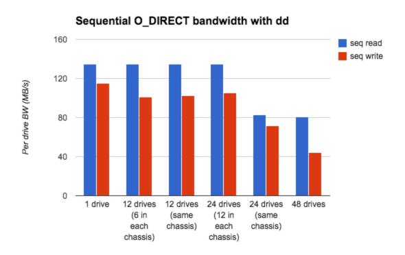
With this baseline we can calculate a maximum OSD write throughput of the entire cluster (assuming co-located OSD journals, single replica, and no other bottlenecks): 150 \* 48 drives \*  $43MB/s / 2 = \sim 150GB/s$ .
