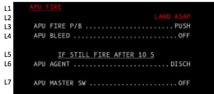
Fig. 6. Example of the display of warning messages on the Warning Display.
