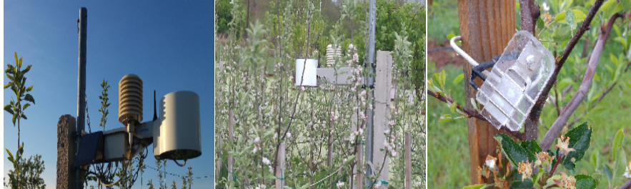
Fig. 3. i-METOS 200 meteorological station and one of the leaf wetness sensors set-up in experimental orchard in Zhegra, Kosovo.
