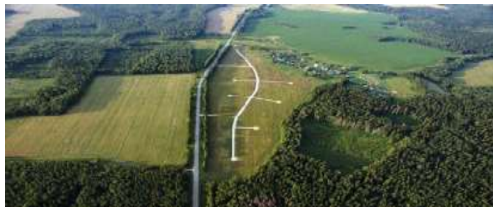
Fig. 4. Vertical shooting - shooting at nadir with an angle to the surface from 87° to 90°
