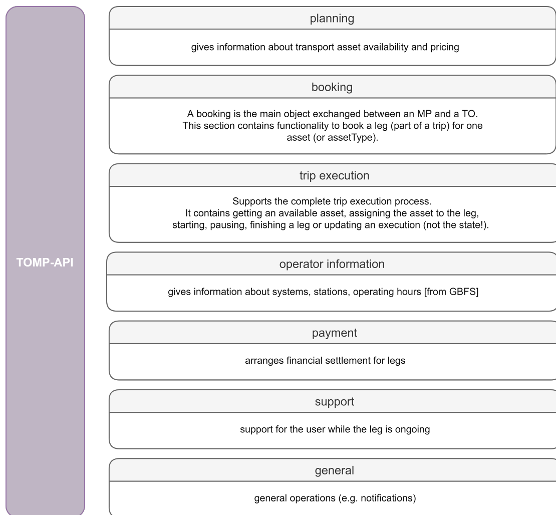
Figure 3: Summary of TOMP-API endpoint categories. For the full API documentation, refer to https://app.swaggerhub.com/apis-docs/TOMP-API-WG/transport-operator_maas_provider_api/1.4.0
