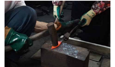
Forging a knife by heating then repeatedly striking iron
