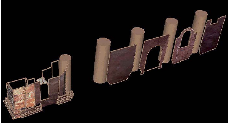
Figure 58 The final model of the West Corridor. Errors in the algorithm solution prevented the modeling of individual stones in the back segments of the hallway. Also, because the photos taken of the back hallway were underexposed, associated texture maps look dark and blurry.
