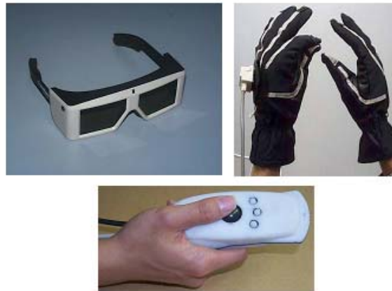
Figure 25 (top) Figure showing a Cave Immersive Virtual Reality environment where a three-dimensional model can be presented in a manner that simulates reality. This is achieved by stereoscopic projections of the scene on the three walls and floor of the cave. The user wears tracked shutter glasses and the model is continuously rendered for his/her perspective. In order to navigate and interact with the scene a wand and pinch gloves are provided that allow users to address commands to the system by finger movements.
