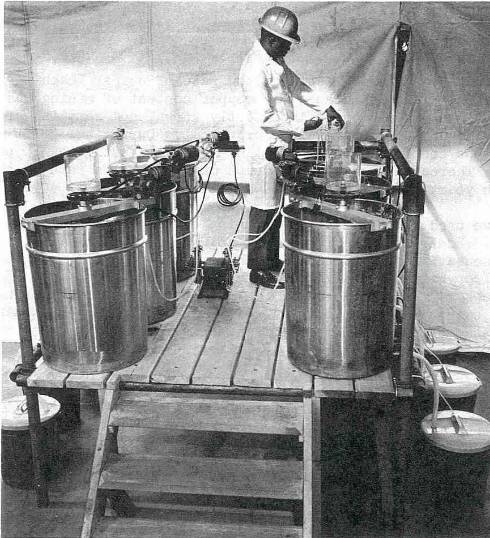
Figure 4.37-6. Percolation leaching of copper waste (Rosenbaum and McKinney 1970, Figure 1).
