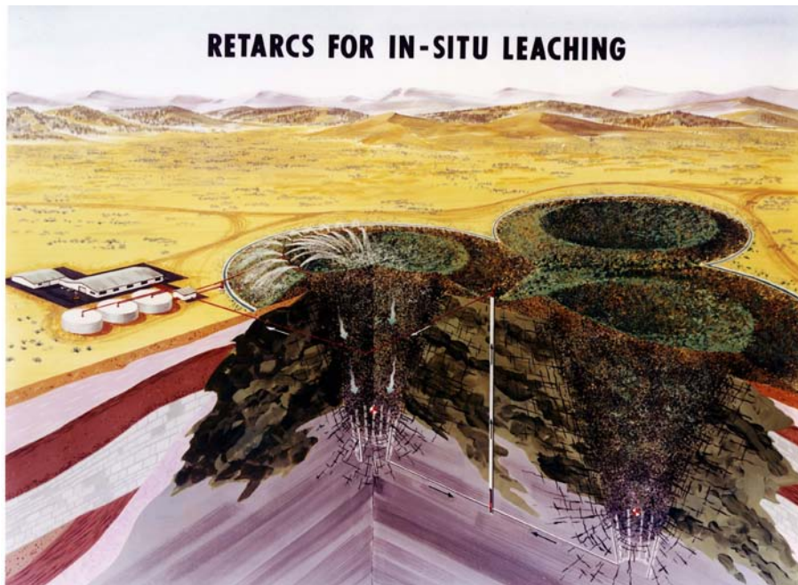
Figure 4.12-2. Conceptual diagram of in situ leaching of a near surface deposit after being fractured by nuclear explosives using the retarc method (Lawrence Livermore National Laboratory n.d.).
