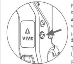
Press and hold the down button to reset the encoder to zero
