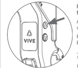
Press and hold the up button to check the firmware version
