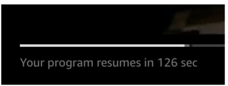
The elements in the client-side tracking metadata that play a role in the ad countdown timer are startTime, startTimeInSeconds, duration, and durationInSeconds. The player uses this metadata, along with the session's elapsed time that it tracks separately, to determine when to display the timer and the value it should be counting down from.
