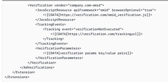
MediaTailor extracts the AdVerifications data from the <Extensions> node and places it into the adVerifications array in the client-side tracking response.
