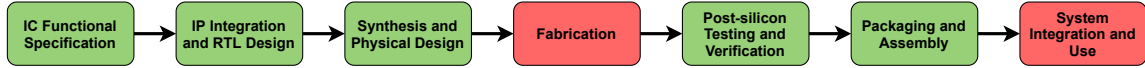
Fig. 1. Design flow and threats. Green stages are secure and Red stages are vulnerable to attacks.
