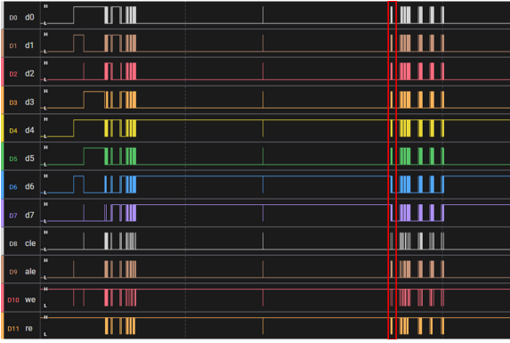
(a) Communication between the flash memory controller and flash memory in the eMMC
