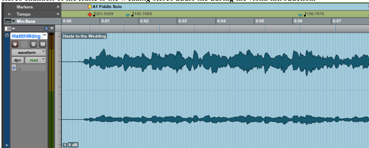
Figure 5.16: Screenshot taken from the Pro Tools session file illustrating the balance of the left and right stereo channels of the Haste to the Wedding stereo audio file during the violin introduction.
