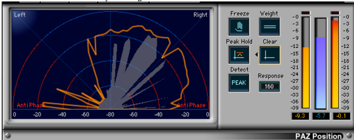
Figure 5.6: Screenshot of Wave's PAZ Position analyser plug-in inserted on the Buachail on Eirne stereo audio file in the Pro Tools session file illustrating a visual representation of the mix during the four-bar introduction which leans heavily to the right.
