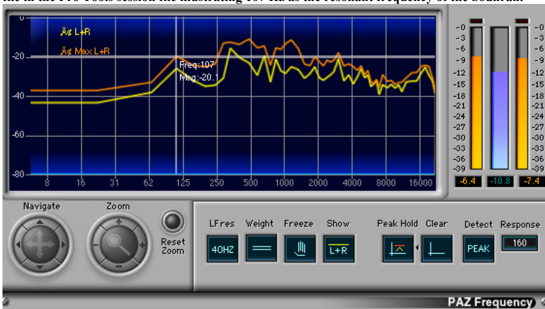
Figure 4.25: Screenshot of Wave's PAZ Frequency analyser plug-in inserted on Toss the Feathers stereo audio file in the Pro Tools session file illustrating 107 Hz as the resonant frequency of the bodhrán.
