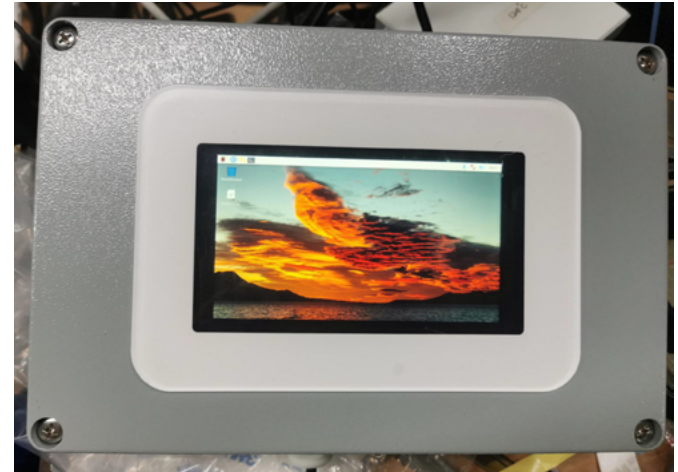
SCADA HMI, Panel PC
