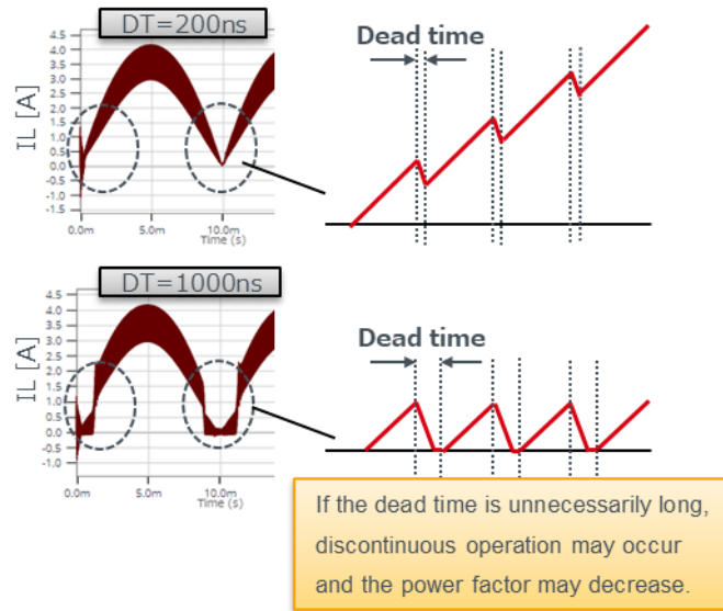
Figure 16. Correlation between Dead Time and Inductor Current I_L
