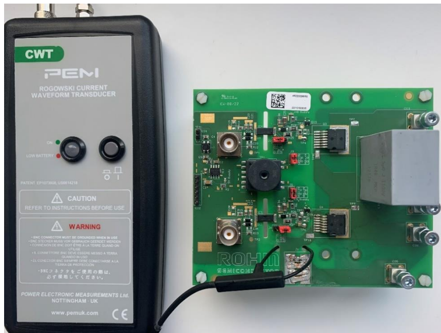
Figure 9: Current measurement set up with Rogowski coil
