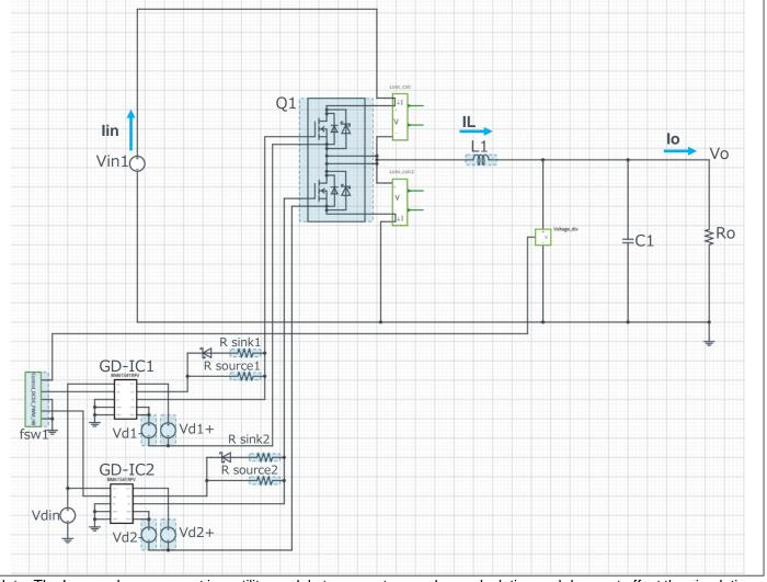
Note: The Loss\_calc component is a utility module to support power loss calculation and does not affect the simulation P. 1 results of circuit operation or performance.
