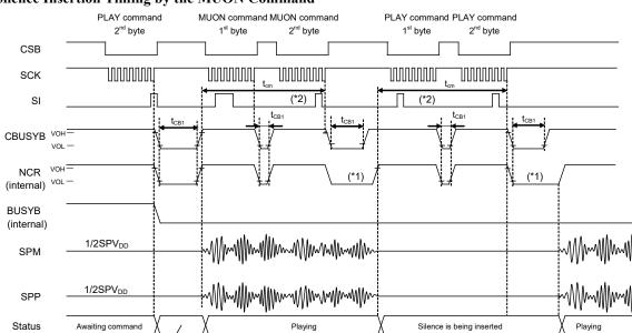
Silence Insertion Timing by the MUON Command
