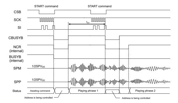
As shown in the diagram above, if continuous playback is carried out, input the START command for the second phrase (tcm) after NCR goes "H". When it cannot, please input the phrase 2 START command after checking that BUSYB became "H"(phrase 1 playback has been finished).
