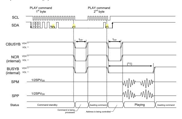
\*1: The maximum length of the "L" interval of BUSYB is  $t_{CB1}$  + voice reproduction time + 12ms.
