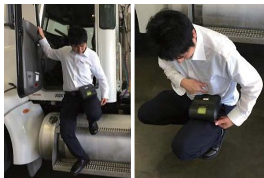
An employee conducting a wearability test of the prototype when getting on and off a customer's delivery truck
