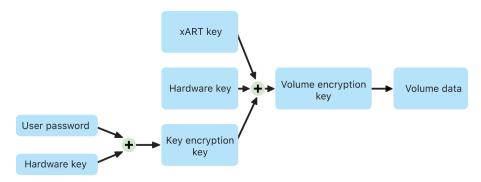
On a Mac with Apple silicon and those with the T2 chip, all FileVault key handling occurs in the Secure Enclave; encryption keys are never directly exposed to the Intel CPU. All APFS volumes are created with a volume encryption key by default. Volume and metadata contents are encrypted with this volume encryption key, which is wrapped with a key encryption key (KEK). The KEK is protected by a combination of the user's password and hardware UID when FileVault is turned on.
