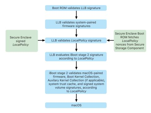
The chip executes code from the Boot ROM in the first step in the chain of trust. macOS secure boot on a Mac with Apple silicon verifies not only the operating system code itself, but also the security policies and even kexts (supported, though not recommended) configured by authorized users.
