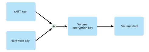
If FileVault is turned on later—a process that's immediate because the data has already been encrypted—an anti-replay mechanism helps prevent the old key (based on hardware UID only) from being used to decrypt the volume. The volume is then protected by a combination of the user password with the hardware UID as previously described.
