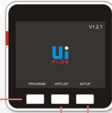
A single press turns on the device A swift double press turns the device off
