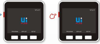
A single press turns on the device A swift double press turns the device off
