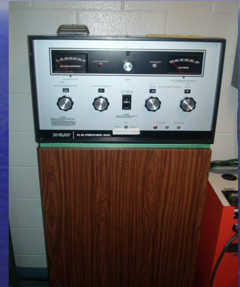
Control panel where the operator can select X-ray ON (exposure) time in fraction of minutes, the energy of X-ray (in kVp) and current applied (higher current = more X-rays).
