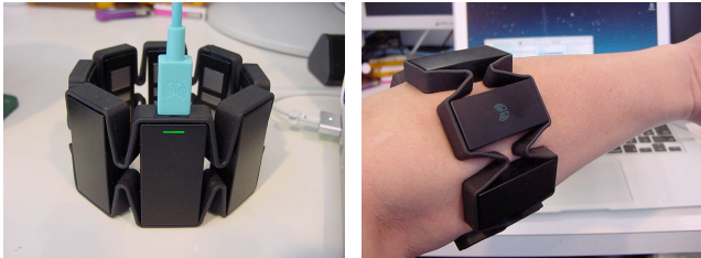
図3 筋電センサ“Myo” Figure 3 “Myo”.
